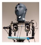
**Figure 1:** The POPEYE robot head is the audio-visual recording device used to acquire the Ravel data set. The color camera pair as well as two (front and left) out of four microphones are shown in the image. Four motors provide for the rotational degrees of freedom and ensure the stability of the device and the repeatability of the recordings.
