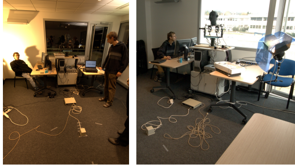
Figure 2: Two viewpoints of the recording environment. The POPEYE robot is in one side of the room to maximize the field of view. As shown, the sequences were shot with and without day light providing for lighting variations. Whilst two diffuse lights were included in the setup to provide for good illumination, no devices were used to modify neither the illumination changes nor the sound characteristics of the room. Hence, the recordings are affected by all kind of audio and visual interferences and artifacts present in natural indoor scenes.
