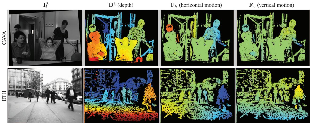
**Fig. 4.** Results on real data. Color-coded disparity and optical flow maps. For disparity  $D^1$ , warmer colors are closer to the camera. For horizontal  $F_h$  and vertical  $F_v$  flows, green color is zero motion, warmer colors is left and up motion, colder colors is right and down motion respectively. Black color denotes unmatched pixel. The figure is best seen in the electronic version.
