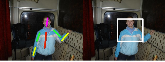
Fig. 3. Example of an annotated image from the ETHZ PASCAL Stickmen dataset. Left: the original stickman annotation. Right: the common reference frame we derived from the sticks.
