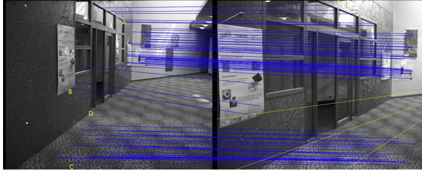
Figure 4: Loria corridor . Nearest neighbour matching, followed by epipolar RANSAC. Correct correspondences can be seen on the walls, and a large number of false ones on the carpet. The epipolar lines in the right image associated with points A and B (from the left image) naturally go through the corresponding point. The same holds for point C whose corresponding point in the right image is not correct. However, the camera motion is properly estimated: for example the epipolar line associated with point D actually go through the corner of the doorway in the other image, in spite that no correspondence is detected in its neighbourhood. Here, the correspondences on the carpet are kept because they satisfy simultaneously the nearest neighbour matching and the epipolar constraint.
