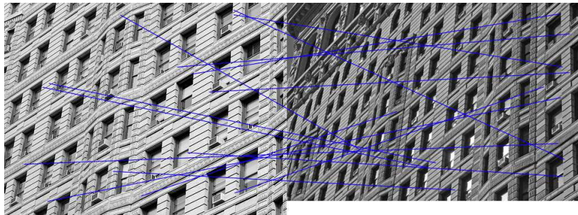
Figure 2: Flatiron image pair. SIFT correspondences (nearest neighbour + distance ratio criterion). It is simply impossible to extract a consistent set of correspondences.
