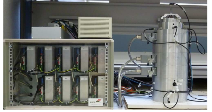
Fig. 4. Magnetic bearing test-bench
