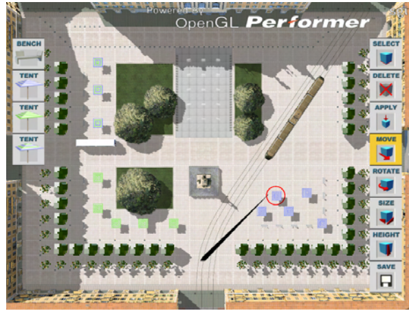
Figure 5: The top view of the VE is displayed with two sets of menus for the insertion and manipulation of dynamic objects. An element (shown with the small circle) is attached to the end of the rod and can be moved and positioned freely.
