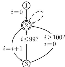
Figure 4: Example: a single loop with break
