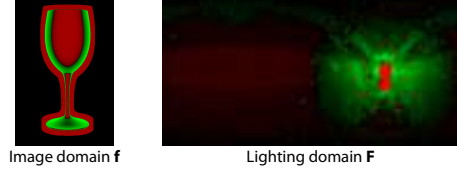
Figure 2: For glass, the image domain weight vector \mathbf{f} is positive (green) along contours and negative (red) in the surrounding regions. In the corresponding lighting domain vector \mathbf{F} the green pixels spread out over a wide area indicating that the contours are lit by a relatively wide region of the environment map.
