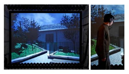
**Figure 2.** Virtual Reality setup. On the left, view of the entire screen in the acoustically damped studio, on the right, a participants equipped with headphones, a head tracker and polarized glasses.
