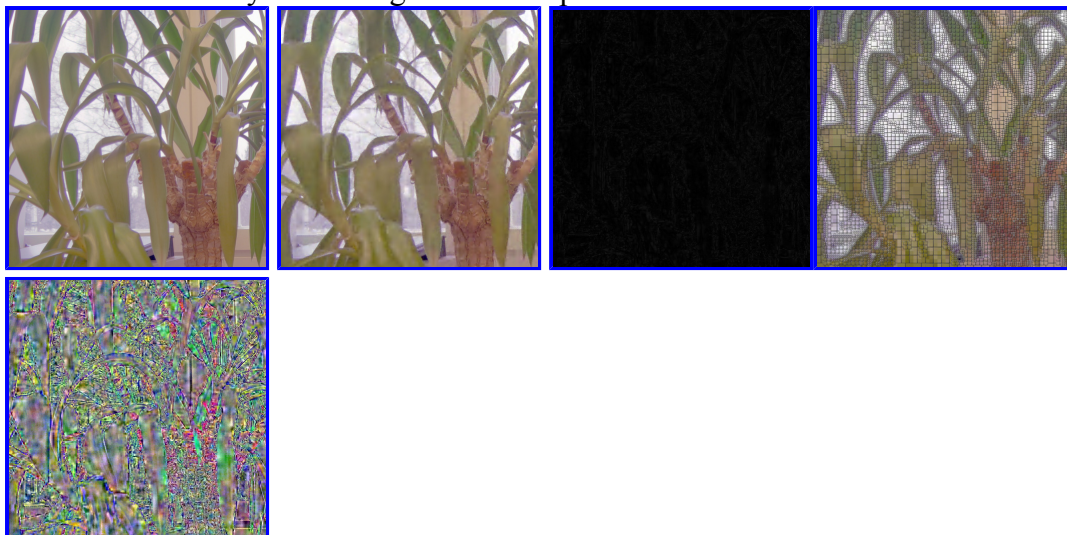
Aggressive tree compression in \log(\text{RGB}) space (input/output/diff/tree) and remaining residuals encoded in a low dynamic range DXT-compressed texture:
