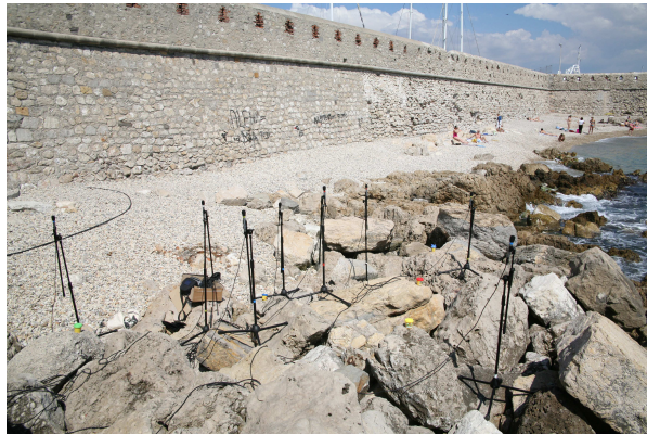
Fig. 9: Recording setup used for the seashore recordings.
