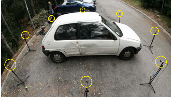
Figure 12: We capture an auditory environment featuring a complex sound source (car engine/exhaust, passengers talking, door slams and on-board stereo system) using 8 microphones surrounding the action.
