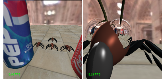
Figure 6: Two images of the ants scene with 8 reflectors. The left image shows a general view of the scene, while on the right we show a close up of the ant eyes showing the distorted scene. This scene runs at 12 fps and contains 30,153 vertices. In the left image the reflected images are very small, but we are computing a full reflection of the scene.
