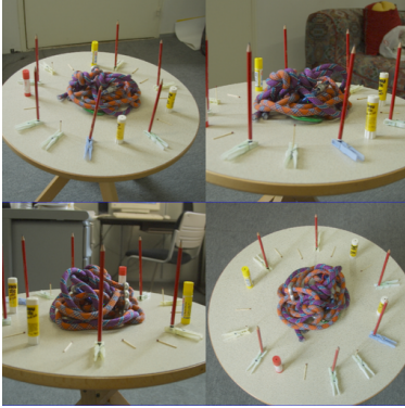
a) 4 of the 14 input images (resolution 2160 \times 1440 ); pencils help the one hour manual calibration with ImageModeler TM [33]
