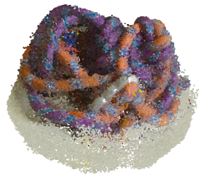
h) Manual generation of more 3D points in user indicated regions during 5 min (total of 115,000 points)
