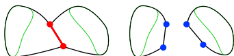
FIGURE 8: Cleanup on thin parts. Each red vertex that is incident to the coinciding red edges is separated in two blue vertices, yielding a surface division in two separate parts.
