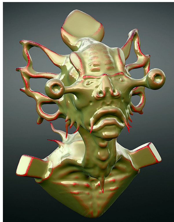
FIGURE 18: Example sculpture created from a sphere by an artist using four tools : sweep deform, inflate-deflate, smooth and trim (for creating flat surfaces). Time taken : 2-3 h. Mesh size : 150k points. Rendering is done with simple shaders as a function of local curvature. This is a real-time capture from the application. d_{detail} for a 1 m statue of the object : 4 mm.
