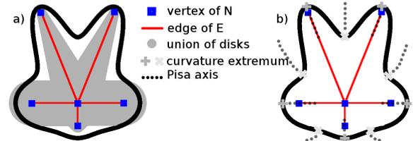
**Figure 3:** Shape representation model. The contour, is the only entity seen by the user. a)  $Sk_c$  and the corresponding union of disks if we consider the topological skeleton associated with  $Sk_c$ . b) detection of all curvature extrema thanks to the branching structure of the skeleton and a gradient technique, and their PISA axes.
