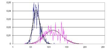
Figure 4: Plots of MoLC-based estimates for the ultrasound image obtained with the GFD model: normalized histograms of the two considered classes and pdf estimates' plots obtained with samples of sizes N = 1862 and N = 218.
