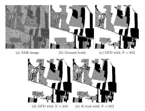
Figure 5: (a) SAR image of flooded area (with learning areas in rectangles) of Piemonte, Italy (COSMO-SkyMed sensor,  $\bigcirc$ ASI), 1000 × 1000 pixels, (b) non-exhaustive ground truth map (white, black, grey - mapped areas, the rest - no ground truth) and supervised classification results obtained with: (c) GFD model on N = 912 samples, (d) GFD model on N = 218 samples and (e) K-root model on N = 912 samples.
