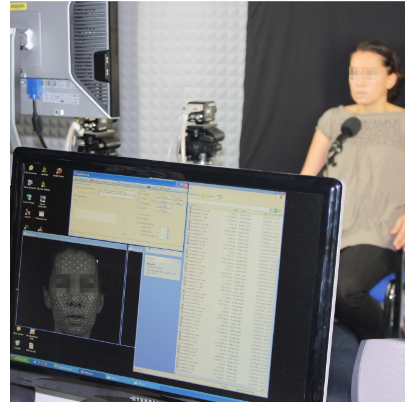
Acoustic-visual data: setup for AV data acquisition; facial marker points are visible in camera array view on foreground display
