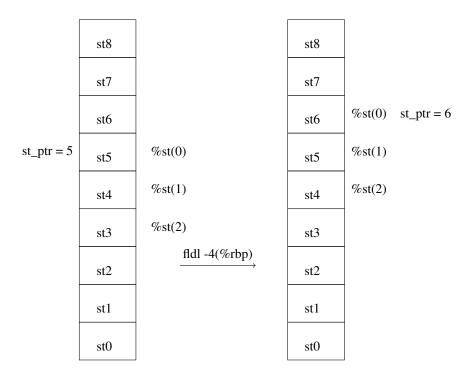
Figure 4.7: Illustration of the stack with instruction *fldl*
