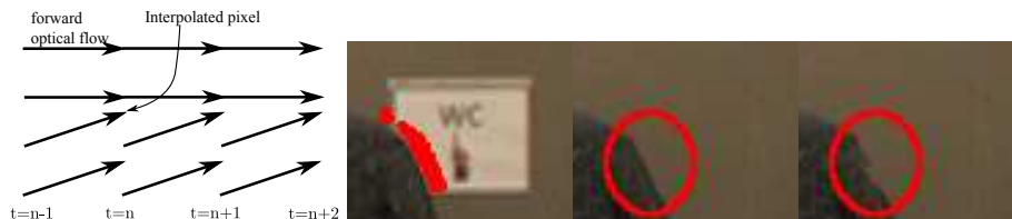
Fig. 3: Results with and without pre-processing of the optical flow. From left to right: a diagram describing the pre-processing, the removed flows, the result obtained using the pre-processed flow and without using it.
