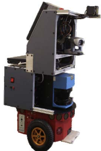
Figure 1: The modified Pioneer P3-DX robot used for the CAROTTE competition.
