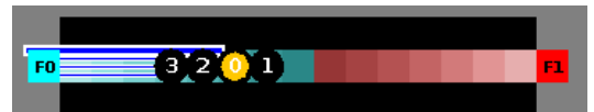
(a) Closest Frontier Allocation : all robots are assigned to the same, closest, frontier
