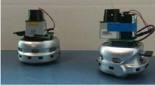
Fig. 11: Two Khepera III (K-Team Corporation) equipped with laser rangefinder (Hokuyo URG-04LX)
