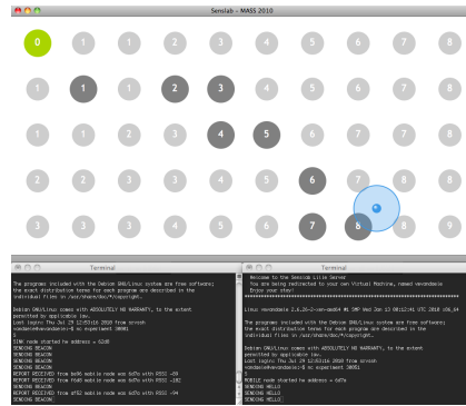
Fig. 7. Demo visualization interface showing routes, messages transmission and mobile nodes location in the upper window, and messages printing on serial links for sink and mobile nodes on lower windows.
