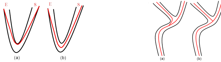
Main centerline using Dijkstra’s algorithm with Euclidian distance (a), the wanted centered centerline (b).
