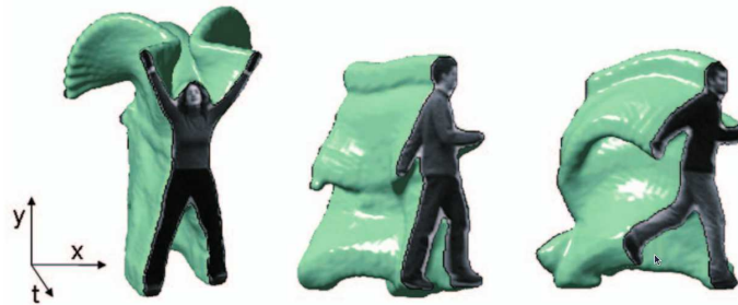
Figure 1.2: Space-time Shapes for “jumping-jack”, “walking”, and “running” actions (courtesy of [BGS + 05]).
