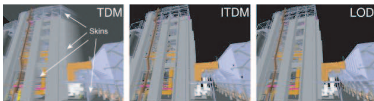
Figure 2.1: A comparison image showing the problems of approaches with a creation based on a fixed viewpoint (TDM) and the incremental textured depth-mesh approach which involves several viewpoints (ITDM). The latter is already very close to results obtained by level of detail methods (LOD), which are much slower, due to the on-the-fly simplification.
