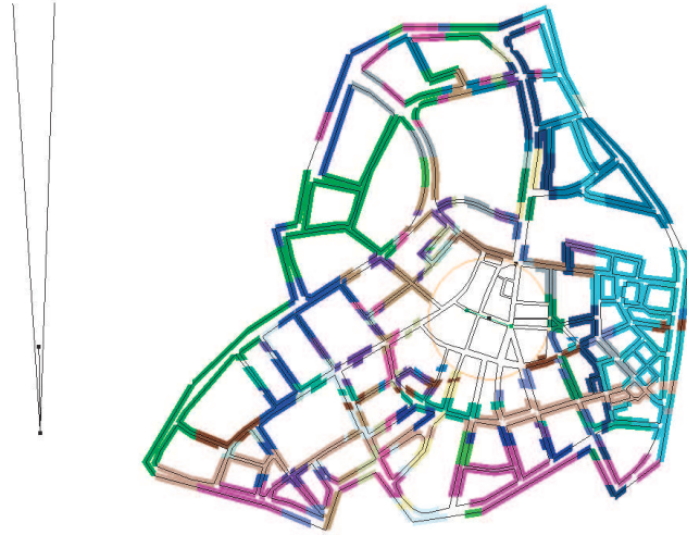
Figure 8.1: A city decomposition on less than 50 Billboards. The view cell corresponds to the green line, the faces inside the red circle where culled. Shown is the decomposition for the first 30 billboards.
