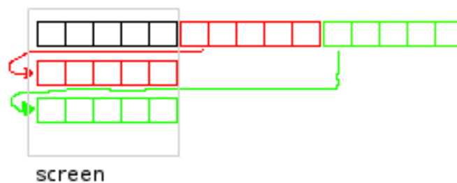
Figure 5.6: A long sampling of the signal is evaluated in 1D, then split into blocks and displayed on screen
