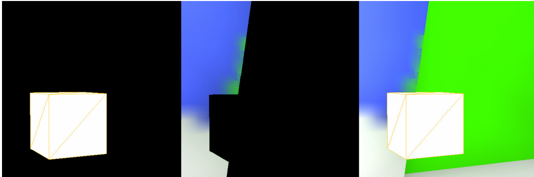
Figure 21 Changing the low quality progressive mode to account for dynamic object occlusion. Render the dynamic object to the frame-buffer (left, before rendering static diffuse surfaces). Account for the dynamic object when rendering the specular index buffer (middle). Final composite (right).
