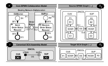
Fig. 3. Graphs for BPMN collaboration and SCA assembly models.
