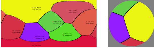
Figure 1: Quantum Voronoi diagram of 1-qubit pure states: Voronoi cells annotated with density matrices on the latitude-longitude map (left) and Voronoi cells visualized on the 3D Bloch sphere (right).
