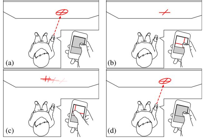
Figure 6: *Laser+Track*. *RayCasting* for coarse pointing (a). Switching to precise mode by touching the surface (b). Controlling cursor movements by moving the thumb (c). Switching back to coarse mode by releasing the thumb (d).
