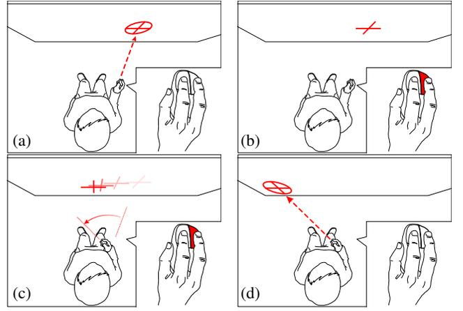
Figure 5: *Laser+Gyro*. *RayCasting* for coarse pointing (a). Switching to precise mode by pressing a button (b). Relative rotational movements control cursor movements (c). Switching back to coarse mode by releasing the button (d). Click performed with left button.
