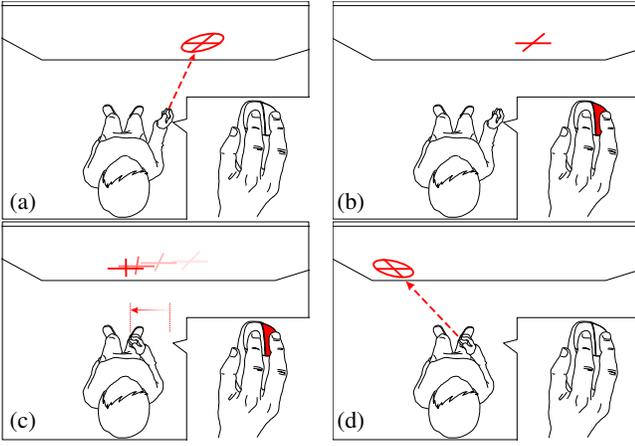
Figure 4: *Laser+Position*. *RayCasting* for coarse pointing (a). Switching to precise mode by pressing a button (b). Relative translational movements control cursor movements (c). Switching back to coarse mode by releasing the button (d). Click performed with left button.
