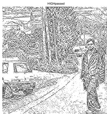
Figure 16. Image passed through a  $10^{th}$  order highpass filter with value of  $\alpha = 1.3$ , sidebands  $40dB$  down.
