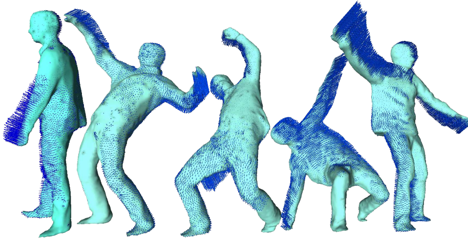
Figure 1: Example of dense scene flow (in blue) from sparse 2D and 3D features and dense normal flow constraints (as for the rest of the paper, figures are best viewed in color).
