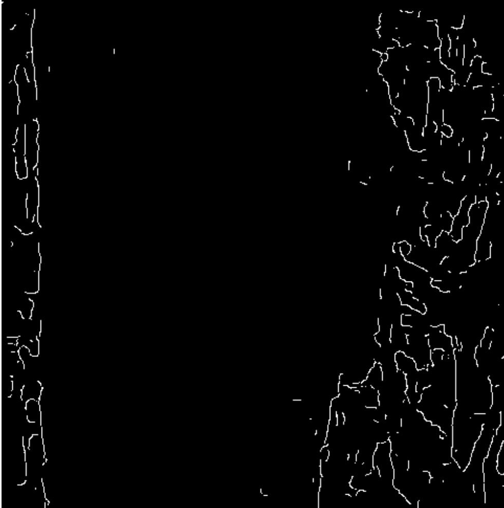
FIG. 25 - Edges obtained from image 22 with Canny's detector, thresholded such that no edges appear in the sea region.
