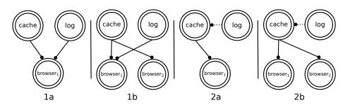
Figure 6: Co-observation in action. 1a) Browser<sub>1</sub> is advised by Cache and Log. 1b) Browser<sub>2</sub> is dynamically created, it should be advised by both aspects but there is an error. 2a) Browser<sub>1</sub> is advised by Cache and Log (as Log co-observes Cache). 2b) Browser<sub>2</sub> is dynamically created, it is advised by both aspects (for Log co-observes Cache).
