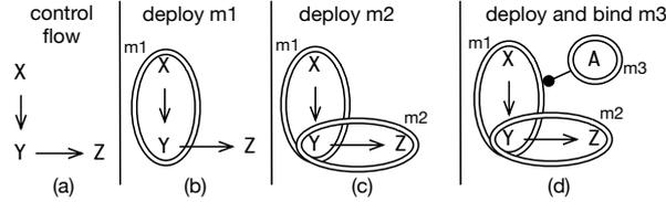
Figure 3: Membranes deployment and aspectual bindings. Membrane  $m_1$  (resp.  $m_2$ ) wraps computation  $X$  and  $Y$  (resp.  $Y$  and  $Z$ ). Membrane  $m_3$  is bound to  $m_1$ : join points from  $m_1$ 's computation will be visible to  $m_3$ 's aspect,  $A$ .
