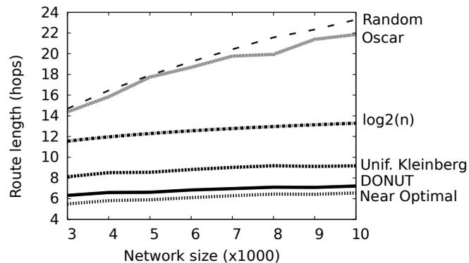
Figure 4: Scalability test: Mean route length in function of the overlay size.
