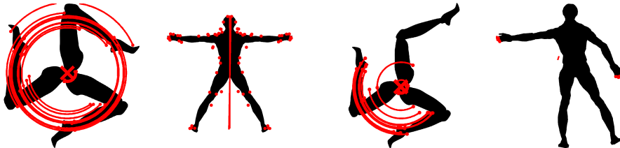
Fig. 5. Performance of the Loy-Eklundh [13] symmetry detection algorithm on our shapes. Left to right: correctly detected rotational C_3 symmetry and bilateral D_1 symmetry, partial C_3 symmetry detection (only one rotation), and incorrect bilateral symmetry detection.
