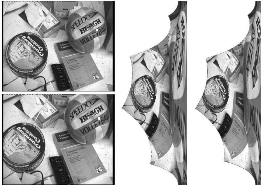
Fig. 6.2 Example of the rectification procedure of Pollefeys et al. On the left, two input images (the epipoles are marked as white dots), on the right the two rectified images. Courtesy of Marc Pollefeys [404].
