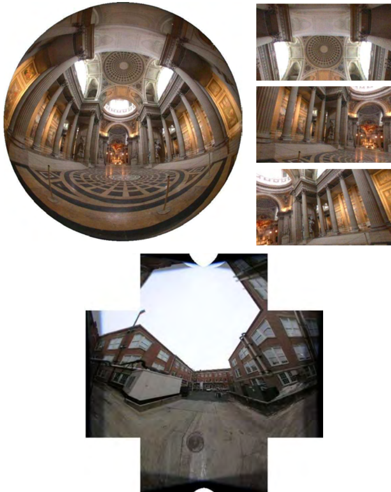
Fig. 6.1 Examples for distortion correction. Left and middle: A fisheye image and distortion corrected sections of it. Right: A cubemap generated from a fisheye image.
