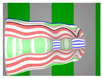
Figure 4. A second synthetic image showing the mirror, the extracted profile, represented in blue, and the used line image, shown in black. Also in this case the image of the visible cross section was not exploited
