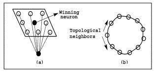
Fig. 1. (a) Lattice Topology employed in conventional **Kohonen-SOM** algorithms. (b) Chain Topology used in **SOM-based** ACMs.
