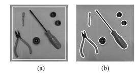
Fig. 11. (a) Image along with initial contour. (b) The converged contours.
