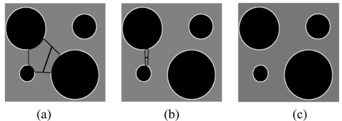
Fig. 10. Continuation of Figs. 9(b) and (c). (a) Contour after second split. (b) Contour after third split. (c) The converged contours.
