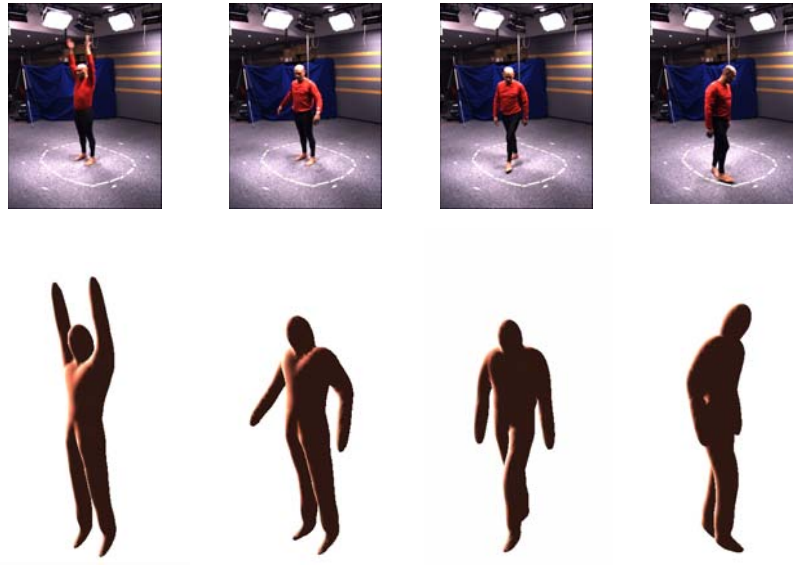
Figure 5: Top: Frames 17, 46, 59, and 81 for one of the six cameras. Bottom: The corresponding pose of the articulated implicit surface shown with the same camera parameters as above.
