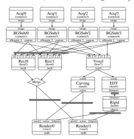
**Figure 10:** FlowVR network graph for the full application graph. Simulations and input device are coupled by FIFO connections. Coherent broadcast greedy patterns (Fig. 4), represented with double horizontal bars, are used on each visualized data as well as on Rec and Rigid inputs.
