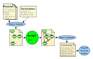
**Figure 2:** The FlowVR application development chain. From modules (left) to the commands the controller forwards to daemons (right).
