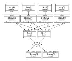
**Figure 9:** FlowVR network graph for FIFO coupling of the mesh reconstruction with the distributed visualization.
