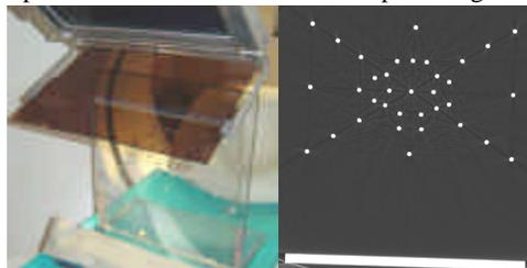
**Fig. 4:** Calibration phantom and its CT image
