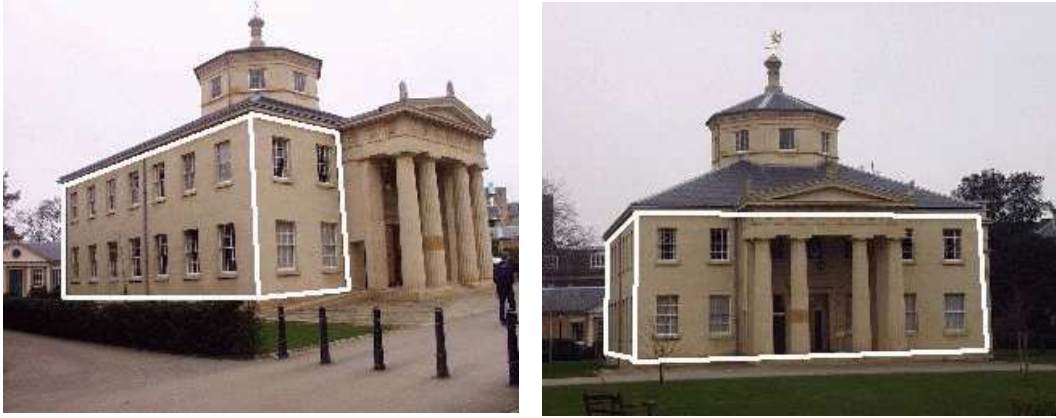
Figure 4: Original pair of photographs taken with different camera zoom setting. Six edges in each image are used to obtain the camera intrinsic parameters and the orientation and position of the viewpoints.
