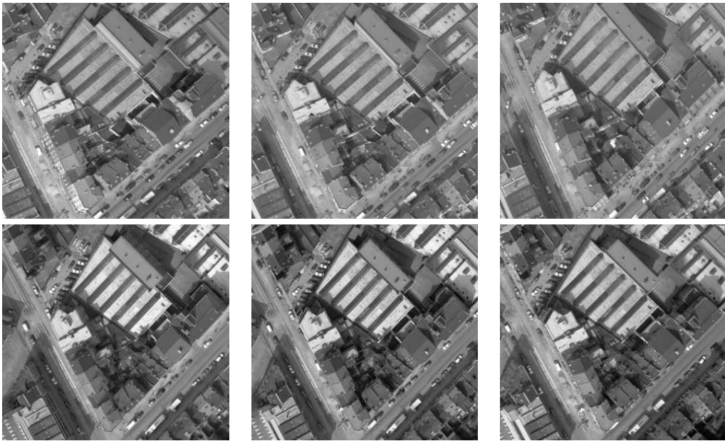
Figure 1: Six overlapping aerial views. The images are about 1200 \times 1200 pixels, one pixel corresponding to a ground length of 8.5cm. The images are acquired at a height of 1300m in two triplets: the camera approximately translated by about 300m between successive views in images 1-3, and between images 4-6. The first set acquired on the outward flight, and the second set on the approximately parallel return flight.
