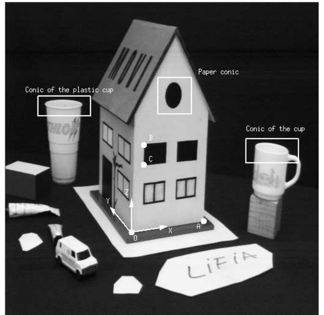
Fig. 3. One of the two original images in which the coordinate system for calibration and the conics used in the experimentation are marked. To have an idea of the real size of the object, OA and BC are measured as 13.75\text{cm} and 2.5\text{cm} .
